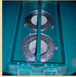
Access to the filter compartments from clean air side
